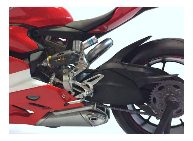
The foot peg assemblies and brackets can be fitted when most of the bike has been assembled.
